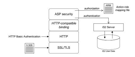
Figure 9: HTTP-Compatible Binding Security Layers
