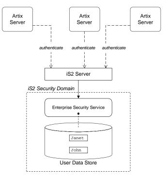
Figure 19: Architecture of an Artix security domain
