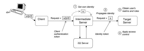
Figure 14: Three-Tier CORBA System Using CSIv2
