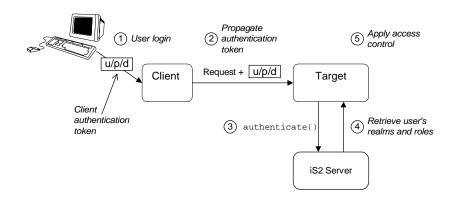
Figure 13: Two-Tier CORBA System Using CSI Credentials
