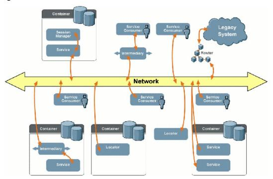
Figure 2.1. Artix ESB and the Virtual Bus
