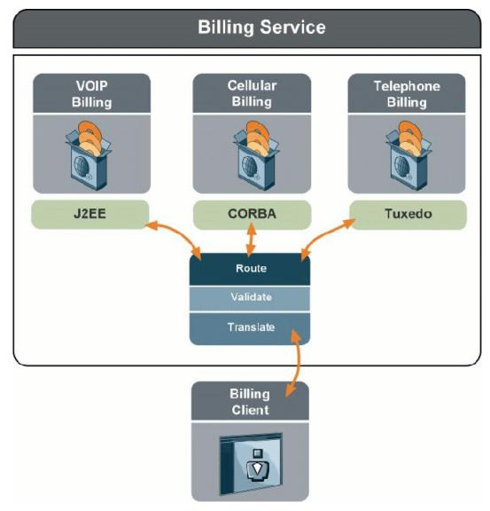
Figure 1.1. Billing System SOA with an ESB
