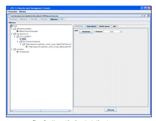
Figure 3: Managed Bus Operation in JConsole
