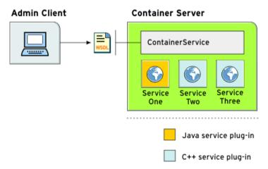
Figure 4: Artix Container Architecture
