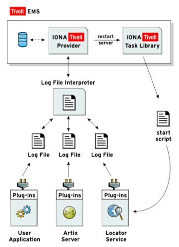
Figure 1: Overview of an Artix and IBM Tivoli Integration
