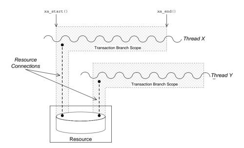
Figure 21: Database Resource Operating in Multi-Threaded Mode
