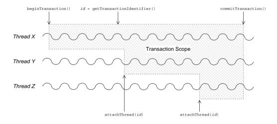
Figure 13: Attaching a Transaction to Multiple Threads
