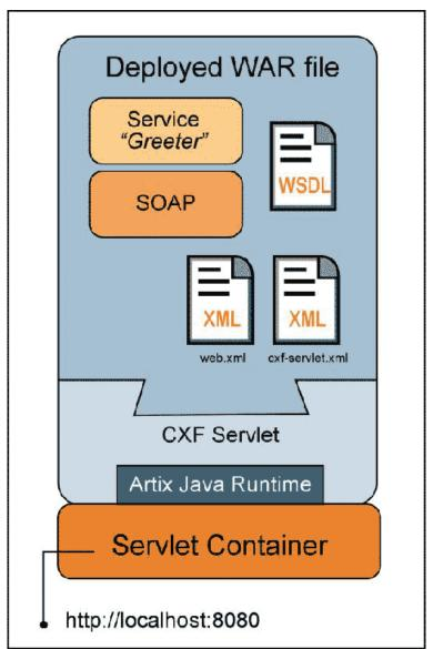
Figure 3. Artix ESB Endpoint Deployed in a Servlet Container
