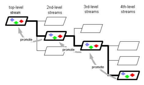
For example, after initial development work on a set of files is completed, the files are submitted to unit testing, then to internal system testing, then to external system ("beta") testing, then to final production. If this workflow is too elaborate for your organization, or not elaborate enough, just design your stream hierarchy differently. You can redesign a project's workflow at any time by changing the stream hierarchy.
