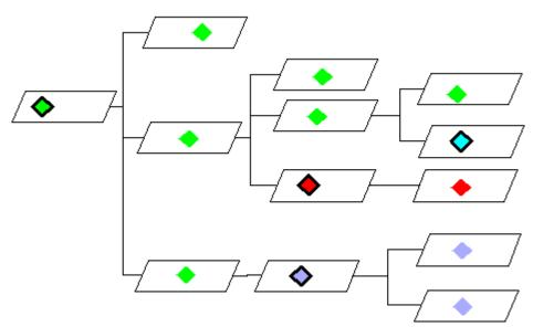
This scheme makes it easy for an organization to manage many development tasks concurrently, each with its own software configuration in a separate stream. As changes are made for certain tasks, AccuRev takes care of automatically applying the changes to the software configurations used by other subsidiary tasks — except for the tasks that are actively working on the same file(s). Just a few *promote* operations can effectively propagate versions to tens or even hundreds of other streams.
