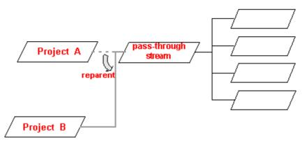
The intermediate stream level doesn't impose any extra day-to-day work on the programmers. The versions they promote automatically pass through the intermediate stream to the project stream.
