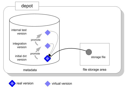
AccuRev distinguishes between the original version, created by a *keep* operation, and all the additional versions created by a *promote* operation:
