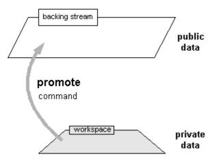
A stream is a configuration of a depot. A typical stream has new versions entering it all the time. Some of the versions are promoted from the workspaces based on them, as described just above; other versions are inherited automatically from higher-level streams. (See *Inheriting Versions From Higher-Level Streams* on page 16.)
