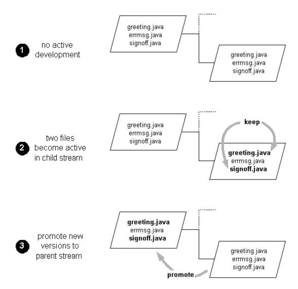
In a multiple-level stream hierarchy, several promotions are required to propagate a set of changes all the way to the top level. Each promotion causes the file(s) to become active in the "to" stream, and inactive in the "from" stream.
