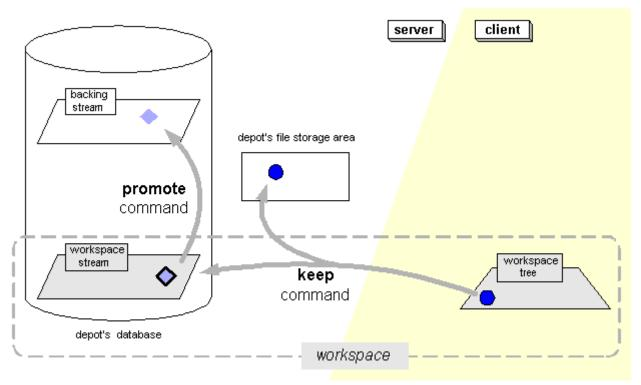
This diagram shows that in AccuRev's client-server world, a workspace has one foot on each side of the divide:
