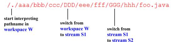
Chaining works correctly if each switch to the next link in the chain occurs at the same pathname component or at a lower component. But here's a situation that violates this rule:
