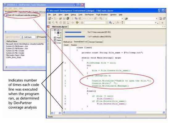
Figure 3-1. Example of Coverage Analysis with a Fault Simulation in Visual Studio
