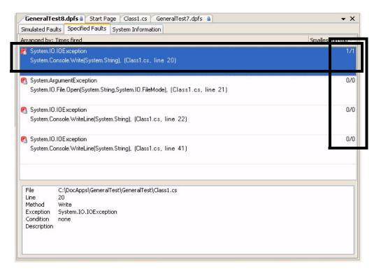
Figure 6-13. Shows that the SystemIO.IOException Was Successfully Simulated
