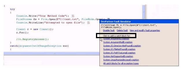
Figure 8-4. Detection of Catch Blocks That Should Be Inserted In the Source Code
