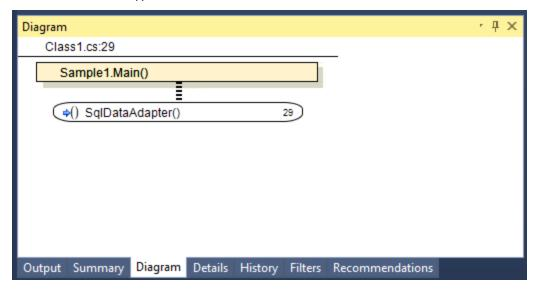
For dataflow issues, the trace starts with the first function to call the taint source, then traces the calls to the source (blue node), and ends the trace at the sink (red node). In the diagram, the source (src) and sink nodes are also labeled. A red X on a vertical axis indicates that the function called finished executing.
