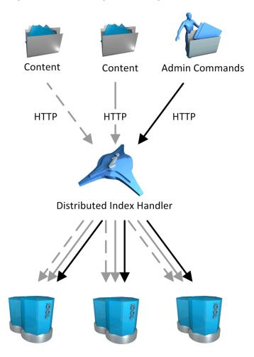
The DIH sends all the index data that it receives (represented by gray arrows in the previous diagram) to all the connected IDOL Servers. The IDOL Servers are exact copies of each other, and must all have the same configuration.
