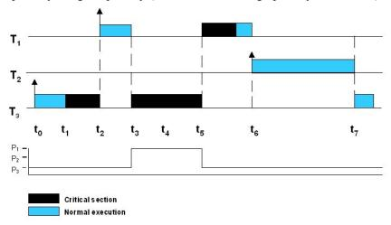
**Figure 9 Priority Inheritance Protocol to Bound Priority Inversion**
