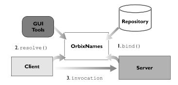
Figure 7: The OrbixNames Architecture
