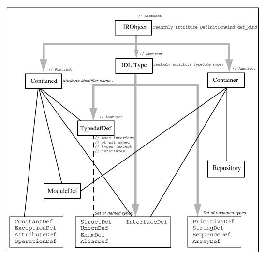
Figure 21: The Hierarchy for Interface Repository Interfaces
