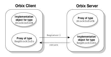
Figure 25: Client Passes Implementation Object Reference to Server
