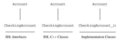
Figure 17: IDL and Corresponding C++ Class Hierarchies
