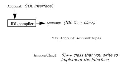
Figure 10: The TIE Approach to Implementing Interfaces
