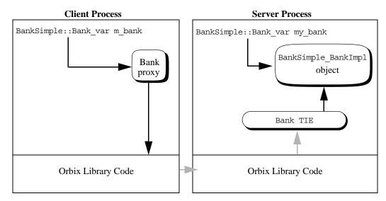
Figure 12: Client Binds to Bank Object (TIE Approach)
