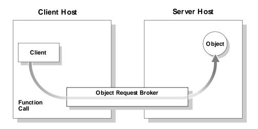
Figure 1: The Object Request Broker
