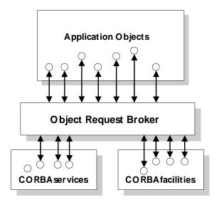
Figure 5: The Object Management Architecture
