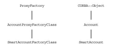
Figure 24: Class Hierarchy for Smart Proxy Class
