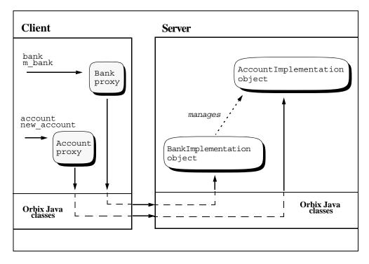
Figure 14: Client Creates Object (ImplBase Approach)
