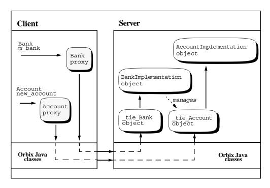
Figure 13: Client Creates Object (TIE Object)
