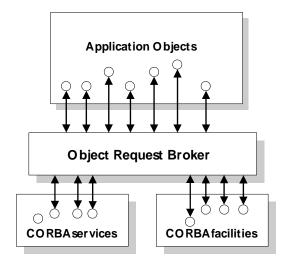
Figure 5: The Object Management Architecture
