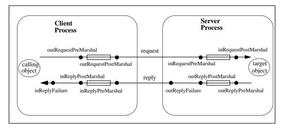
Figure 29: Per-Process Monitor Points
