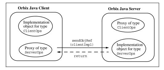
Figure 20: Client Passes Implementation Object Reference to Server
