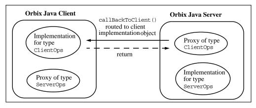
Figure 21: Server Invokes Operation on Client's Callback Object
