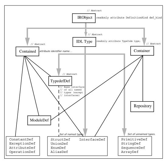
Figure 26: Hierarchy for Interface Repository Interfaces
