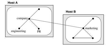
Figure 16: Naming Graph Spanning Different Name Servers
