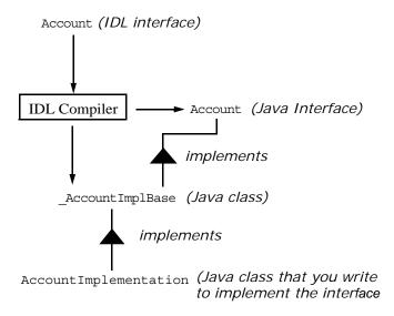
Figure 12: The ImplBase Approach to Defining an Implementation Class
