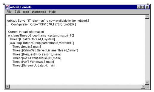
Figure 24: Sample Output from Tools -> Threads Menu Option
