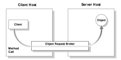
**Figure 1:** The Object Request Broker
