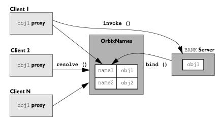
Figure 4: Example of Typical OrbixNames Usage
