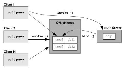
Figure 9: Example of Typical OrbixNames Usage
