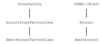
Figure 17.1: Class Hierarchy for Smart Proxy Class
