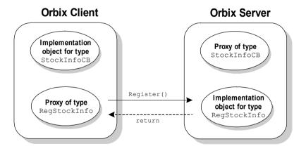
Figure 18.1: Client Passes Implementation Object Reference to Server
