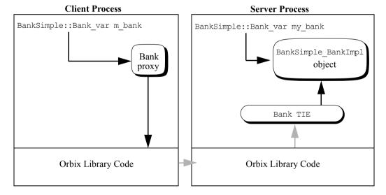
Figure 5.4: Client Binds to Bank Object (TIE Approach)
