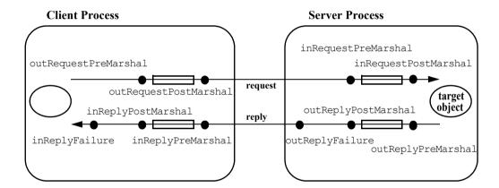
Figure 16.2: Per-process Monitor Points
