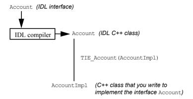
Figure 5.2: The TIE Approach to Implementing Interfaces
