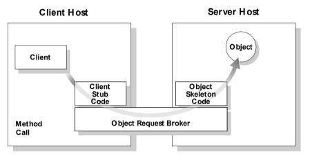
Figure 1.2: Invoking on a CORBA Object
