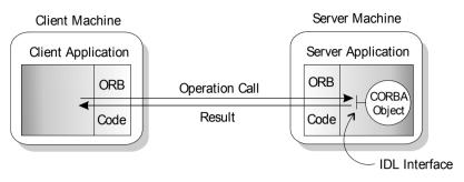
Figure 2.1: Client Making a Single Operation Call on a Server
