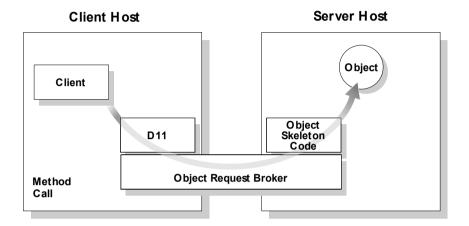
Figure 1.3: Client Invoking a Method Using the DII
