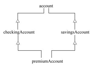
Figure 5.1: Multiple Inheritance of IDL Interfaces
