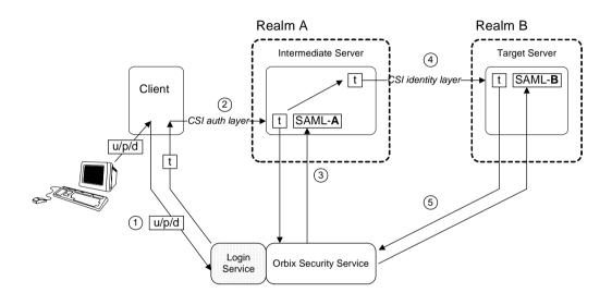
Figure 28: Intermediate and Target Belong to Different Realms
