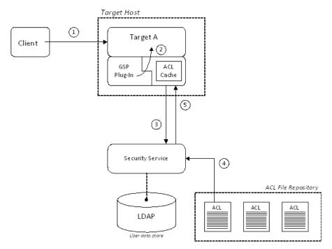
Figure 37: Centralized ACL scenario
