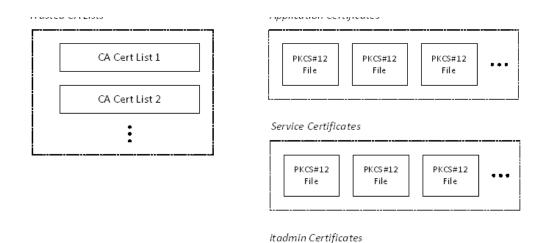
Figure 47: Overview of Certificates in a Typical Deployed System
