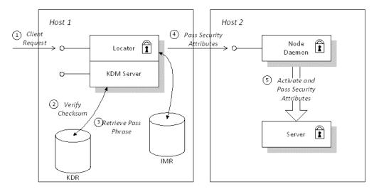
Figure 61: Automatic Activation of a Secure Server
