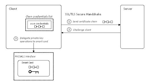
Figure 15: Using PKCS#11 Credentials to Authenticate a Client to a Server
