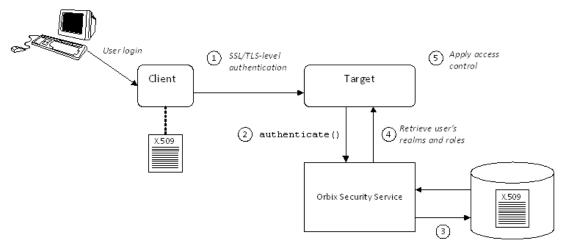
Figure 19: Overview of iSF Certificate-Based Authentication
