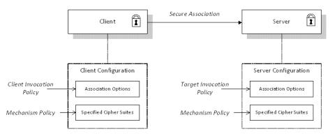
Figure 52: Configuration of a Secure Association
