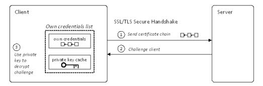
Figure 13: Using PKCS#12 Credentials to Authenticate a Client to a Server
