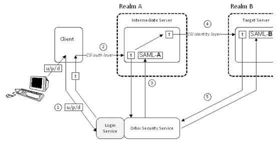
Figure 28: Intermediate and Target Belong to Different Realms
