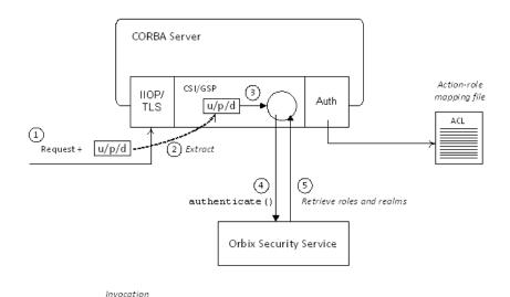
Figure 65: CSIv2 in the Orbix Security Framework
