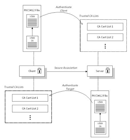
Figure 55: Target and Client Authentication
