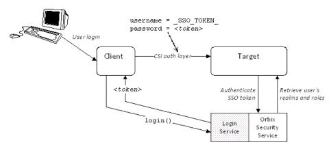
Figure 25: Overview of Certificate-Based Authentication with SSO
