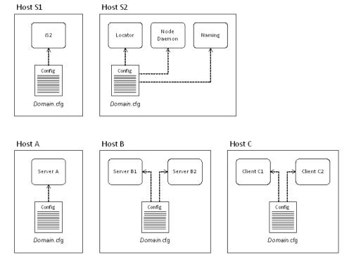
Figure 39: Overview of a Secure File-Based Domain
