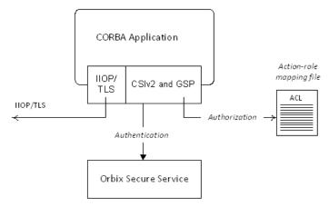
**Figure 16:** A Secure CORBA Application within the iSF
