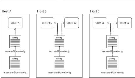
Figure 40: Overview of a Secure CFR Domain
