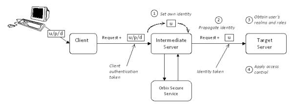
Figure 18: Three-Tier CORBA System in the iSF
