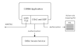
Figure 11: Security Plug-Ins in a CORBA Application
