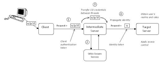
Figure 69: Three-Tier CSI Scenario with Copying of CSI Credentials
