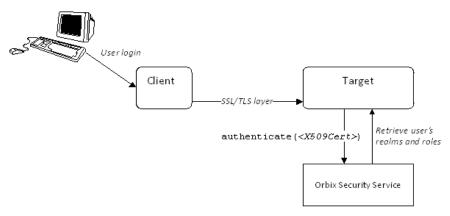
Figure 24: Overview of Certificate-Based Authentication without SSO
