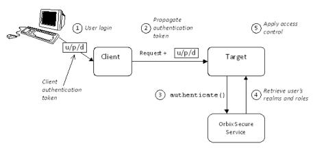
**Figure 17:** Two-Tier CORBA System in the iSF
