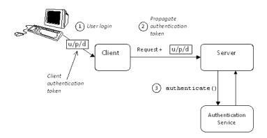
Figure 63: Basic CSIv2 Authentication over Transport Scenario
