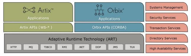
Figure 1: ART Plug-In Architecture
