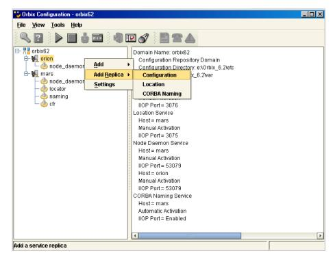
Figure 2: Orbix Configuration GUI
