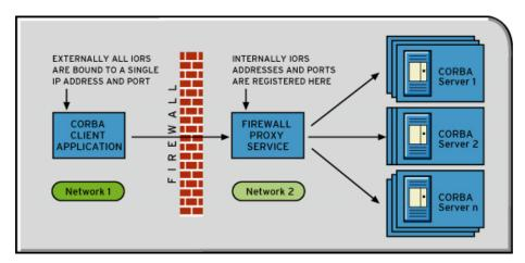
Figure 8: Firewall Proxy Service
