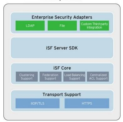
Figure 5: Architecture of the Orbix Security Service, which is designed to integrate with your choice of enterprise security solution.
