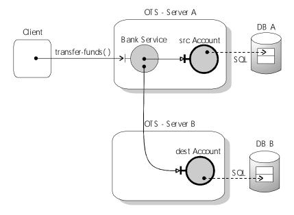
Figure 7.4: Distributed Transaction with Ordinary Client.
