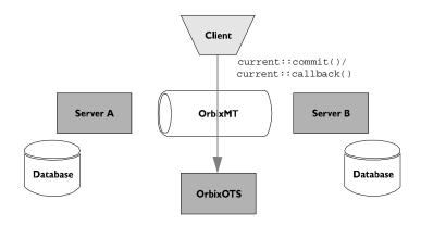
Figure 7.8: Client Ends a Transaction
