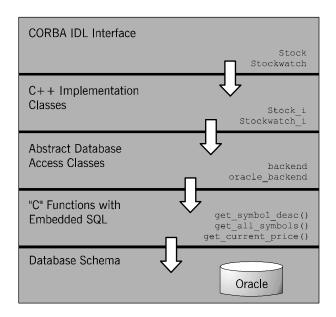
Figure 4.4: Structure of StockWatch Server Program
