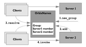
Figure 9.2: Naming Service and Load Balancing
