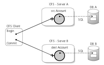
Figure 7.3: Distributed Transaction with OTS Client.
