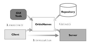
Figure 1.7: The OrbixNames Architecture
