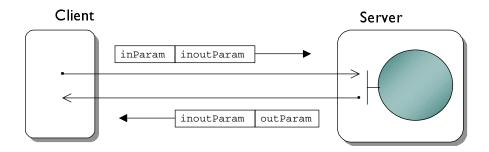
**Figure 3.1:** Parameters Passed as Foo::op() is Invoked.
