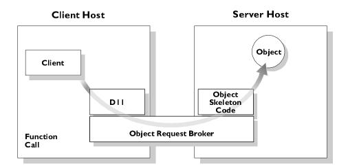
Figure 1.3: Client Invoking a Function Using the DII
