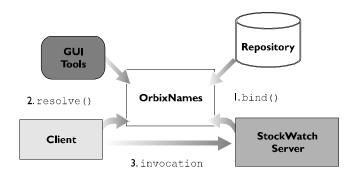
Figure 5.1: Using OrbixNames in Orbix
