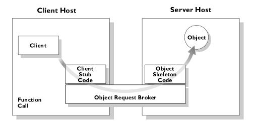
Figure 1.2: Invoking on a CORBA Object
