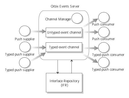
Figure 6.3: Architecture of the OrbixEvents Server.
