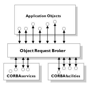
Figure 1.5: The Object Management Architecture
