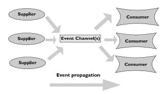
Figure 1.8: Schematic View of OrbixEvents Architecture
