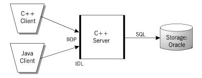
Figure 4.3: Simple Three-Tiered Architecture
