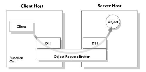
Figure 1.4: Function Call Using the DII and DSI
