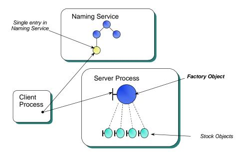
Figure 4.2: Factory Object—One Object Published in the Naming Service
