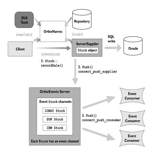
Figure 6.5: The Architecture of StockWatch When Using Events
