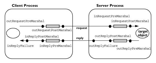
Figure 16.2: Per-process Monitor Points
