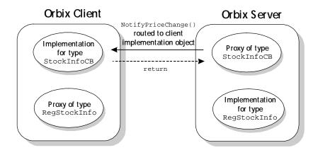
Figure 18.2: Server Invoking Operation on Client Callback Object
