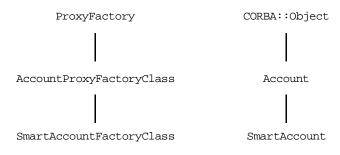
Figure 17.1: Class Hierarchy for Smart Proxy Class
