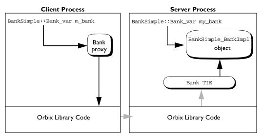
Figure 5.4: Client Binds to Bank Object (TIE Approach)
