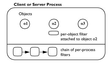
Figure 16.1: Per-process and Per-object Filtering
