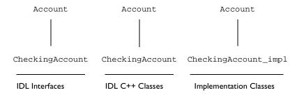
Figure 8.1: IDL and Corresponding C++ Class Hierarchies
