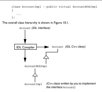
Figure 10.1: Casting From Interface Class to Implementation Class Using the BOAImpl Approach
