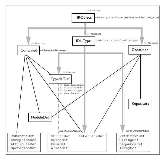
Figure 15.1: The Hierarchy for Interface Repository Interfaces
