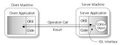
Figure 1.1: Client Making a Single Operation Call on a Server
