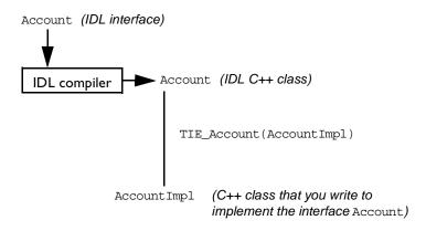
Figure 5.2: The TIE Approach to Implementing Interfaces
