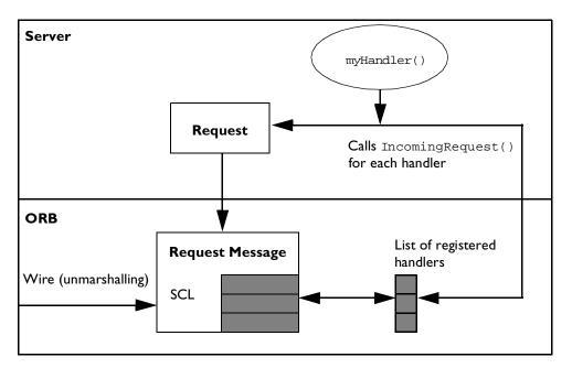
Figure 23.2 illustrates the operation of the service context per-request model on the server side.
