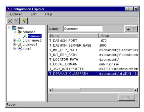
Figure 6.2: Common Configuration Settings
