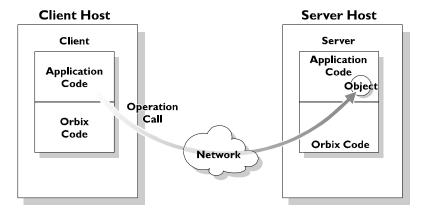
Figure 1.1: An IDL Operation Call on a Distributed Object
