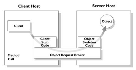
Figure 1.2: Invoking on a CORBA Object
