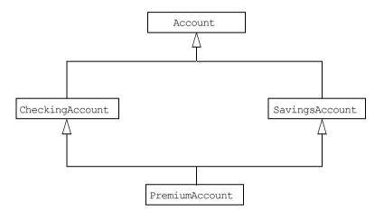
**Figure 10.2:** Multiple Inheritance of IDL Interfaces
