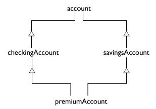
Figure 5.1: Multiple Inheritance of IDL Interfaces
