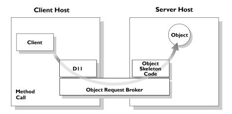
Figure 1.3: Client Invoking a Method Using the DII
