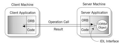
Figure 2.1: Client Making a Single Operation Call on a Server
