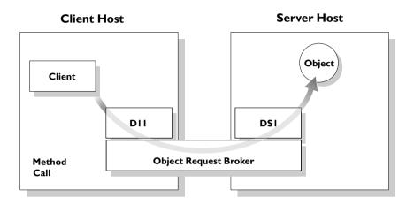
Figure 1.4: Method Call Using the DII and DSI
