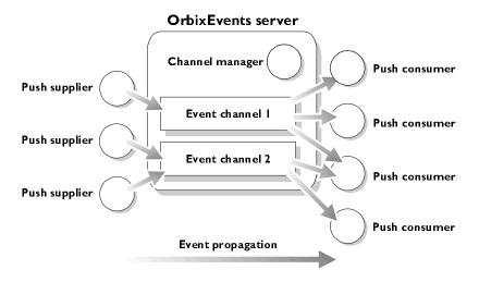
Figure 3.1: Example OrbixEvents Architecture with Two Event Channels
