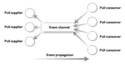
Figure 5.5: Pull Model Suppliers and Consumers Communicating through an Event Channel
