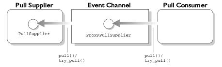
**Figure 6.3:** Transfer of an Event through an Event Channel to a Consumer using the Untyped Pull Model
