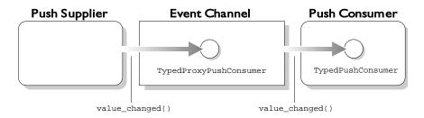
**Figure 6.5:** Transfer of an Event Through an Event Channel to a Consumer Using the Typed Push Model
