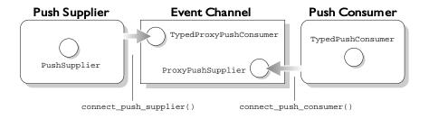
**Figure 6.4:** Push Supplier and Push Consumer Connecting to an Event Channel using the Typed Model
