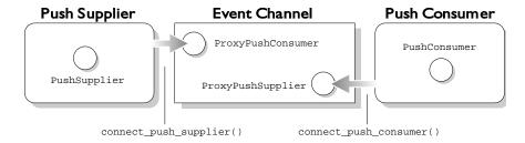
**Figure 6.1:** Push Supplier and Push Consumer Connecting to an Event Channel in the Untyped Model
