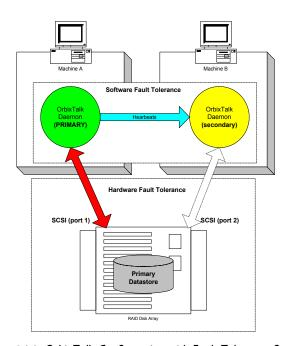
Figure 14.1: OrbixTalk Configuration with Fault Tolerance Supported
