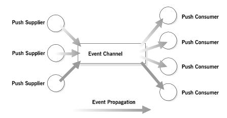
Figure 5.4: Push Model Suppliers and Consumers Communicating through an Event Channel
