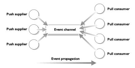
Figure 5.6: Push Model Suppliers and Pull Model Consumers in a Single System
