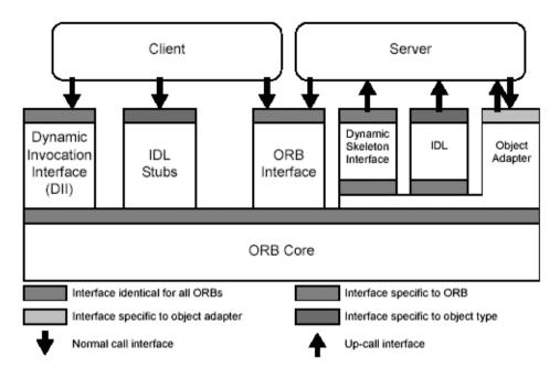
Figure 6: The Components of an ORB
