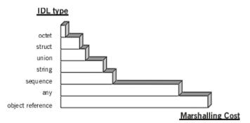
Figure 11: Relative Marshalling Cost of Type of IDL Data Sent
