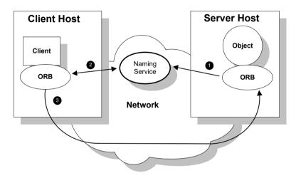
Figure 2: Overview of a Simple Orbix Application
