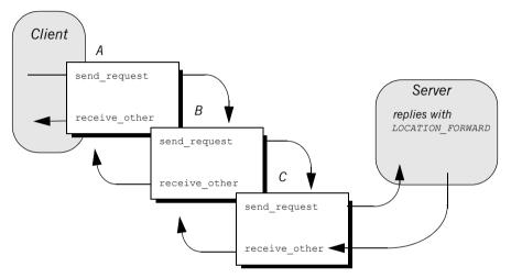
Figure 46: Client interceptors process a LOCATION\_FORWARD reply.
