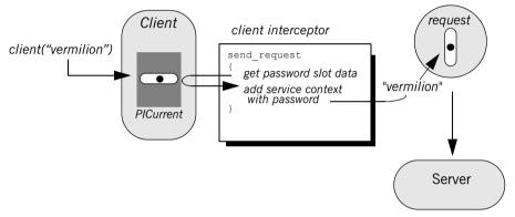
**Figure 44:** *PICurrent facilitates transfer of thread context data to a request or reply.*
