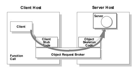
Figure 3: Invoking on a CORBA object
