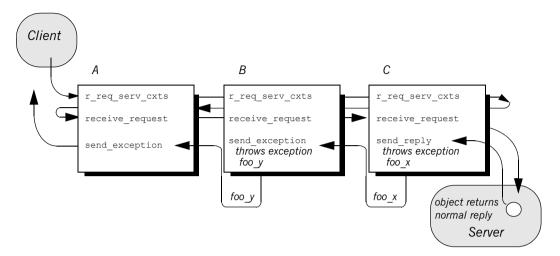
Figure 51: Server interceptors can change the reply type.
