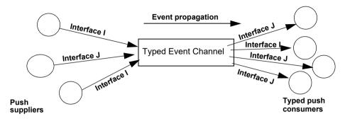
Figure 42: Push consumers pushing typed events to typed push consumers
