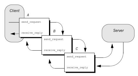
Figure 45: Client interceptors process a normal reply.
