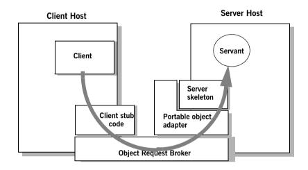
Figure 4: The portable object adapter
