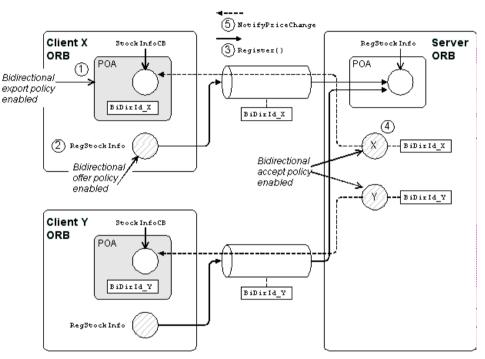
Figure 52: Basic Bidirectional GIOP Scenario—Stock Feed
