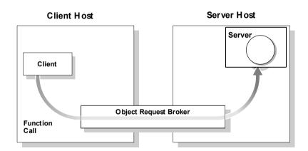
Figure 2: The object request broker
