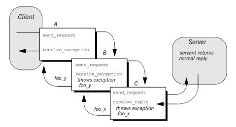
Figure 48: Client interceptors can change the nature of the reply.
