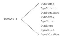
Figure 20: Interfaces that derive from the DynAny interface
