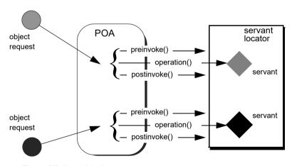
**Figure 17:** The POA directs each object request to the servant locator, which returns a servant to the POA to process the request.
