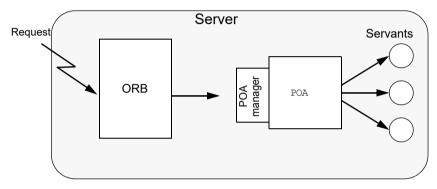
**Figure 11:** The server-side ORB conveys client requests to the POA via its manager, and the POA dispatches the request to the appropriate servant.
