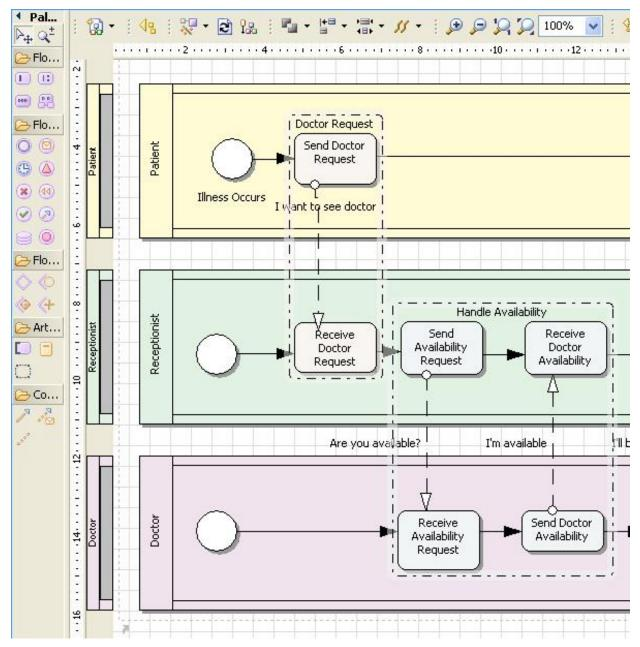
The Group element allows you to easily differentiate between sections of a BPMN diagram. You can easily divide a BPMN diagram into logical parts using the Group element. A Group permanently keeps track of content, resizes on element move, colors elements with selected color, etc.
