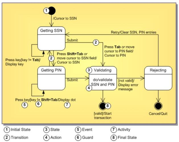
States are depicted as rounded rectangles. Transitions are arrows from one state to another. Events or conditions that trigger transitions are written next to the arrows. This diagram has two self-transitions: Getting SSN and Getting PIN. The initial state (shown as a black circle) is a dummy to start the action. Final states are also dummy states that terminate the action.
