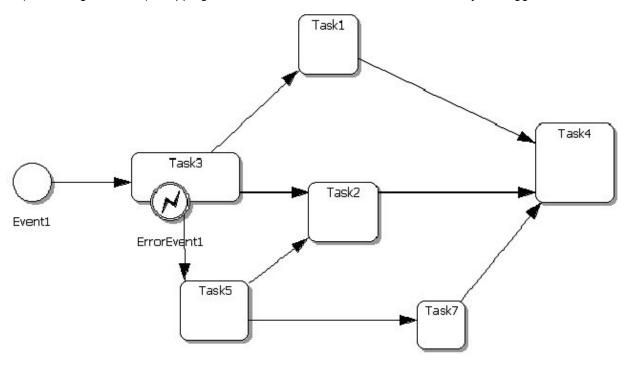
Any task or subprocess with boundary events starts a flow. All the elements from the exception flow or normal flow belong to that flow element, until all the paths from them merge (as in the figure below). If the paths do not merge explicitly, the program assumes that they merge in the end element.
