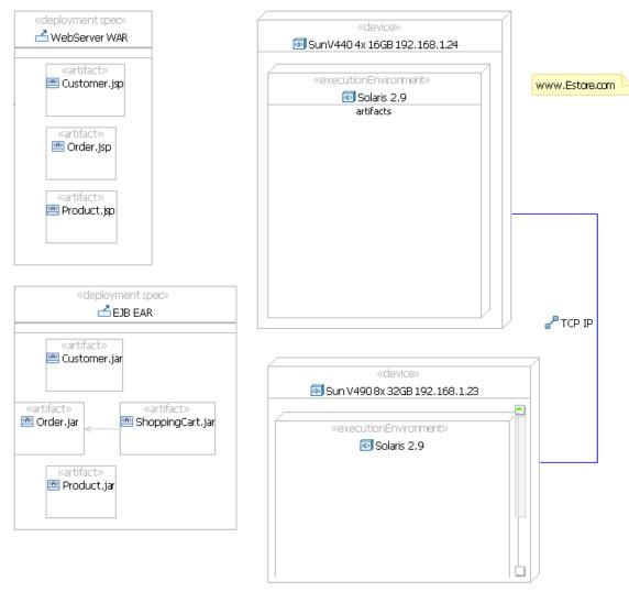
The key elements used in a deployment diagram are nodes, components, and associations. There are two standard stereotypes for nodes: Devices represent physical devices such as a server machine or a workstation, and Environments represent software execution engines such as an Apache Web server, a Tomcat Web container or an Internet Explorer Web browser.
