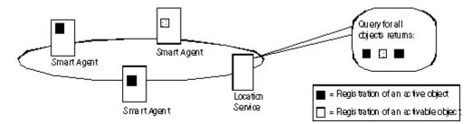
The Location Service can make use of the information the Smart Agent keeps about each object instance. For each object instance, the Location Service maintains information encapsulated in the structure ObjLocation::Desc shown below.
