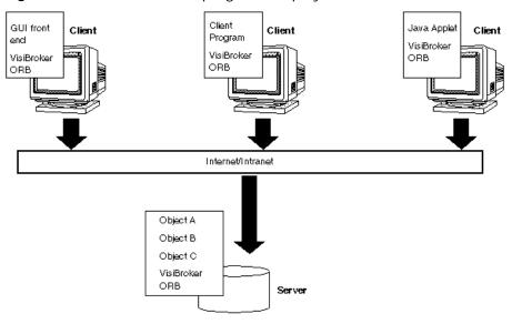
Figure 4 Client and server programs deployed with VisiBroker ORBs
