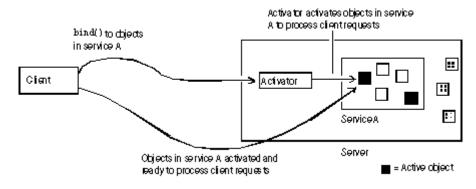
Figure 39 Process of Deferring Activation for a Service
