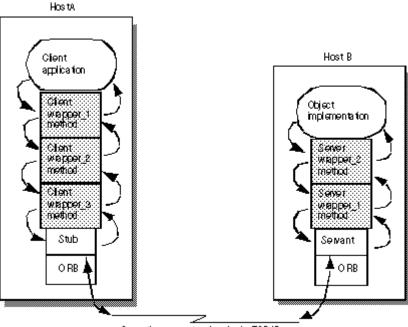
Operation request and reply via TCP/IP
