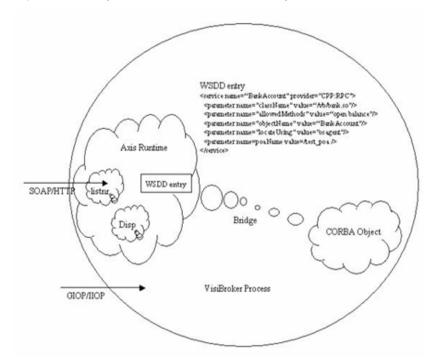
Figure 43 Components inside a VisiBroker process
