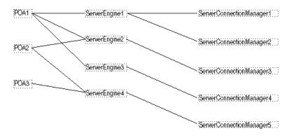
The simplest case is where POAs have their own unique single server engine. Here, requests for different POAs arrive on different ports. A POA can also have multiple server engines. In this scenario, a single POA supports requests coming from multiple input ports.
