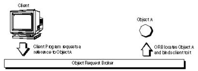
Figure 1 Client program acting on an object
