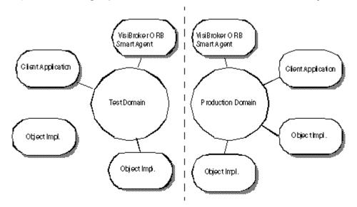
Figure 18 Running separate VisiBroker ORB domains simultaneously
