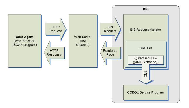
Figure 2-1. BIS Block Diagram.
